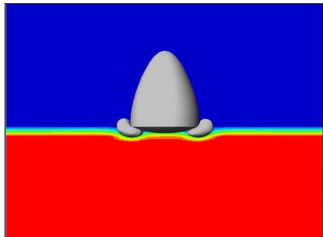
**Figure 7. Generic Spacecraft Water Landing With Inflated Airbags**
