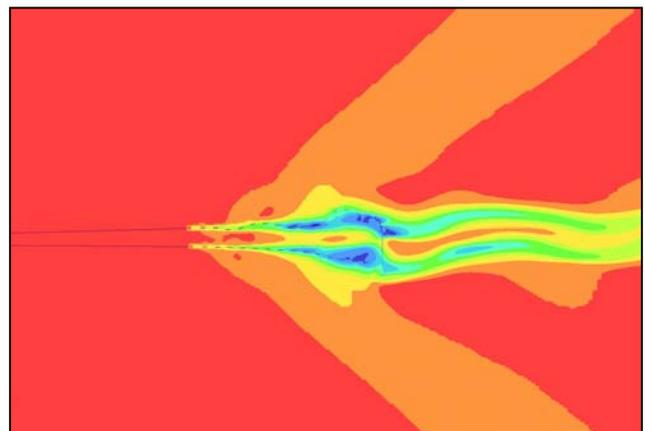
**Figure 17. A Ribbon Parachute with Excessive Geometric Porosity**
