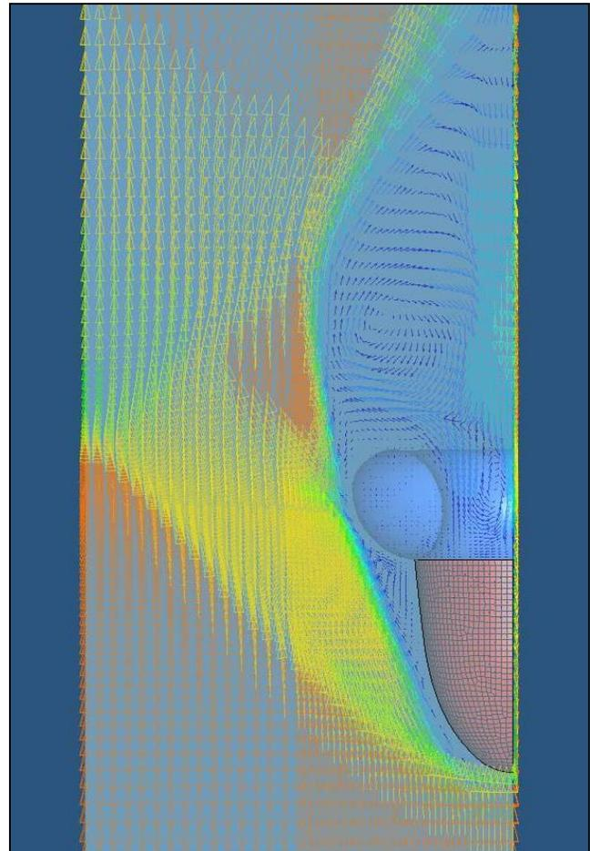
**Figure 19. Flow around a Generic Fore Body and Attached Ballute at Supersonic Mach**
