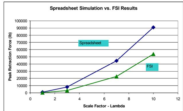
**Figure 14. Multi-body and FSI Results, Classical Treatment of Air Included in the Parachute**
