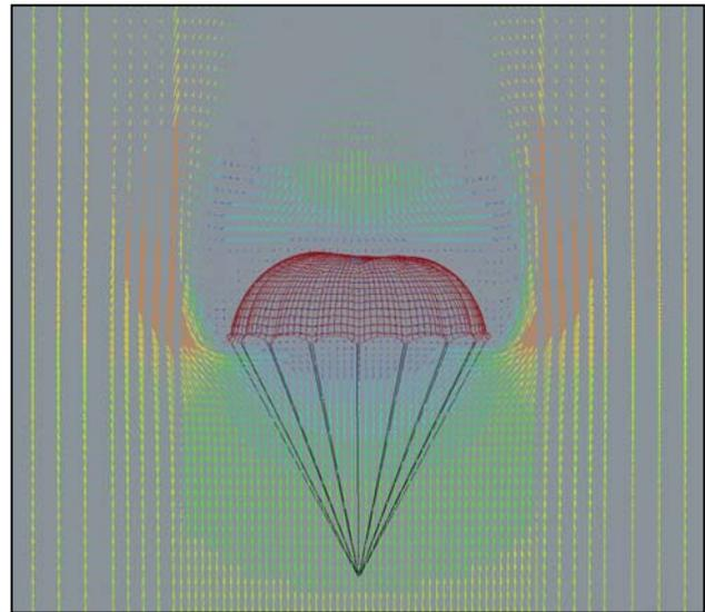
**Figure 11. Beginnings of Non-Symmetric Loading**
