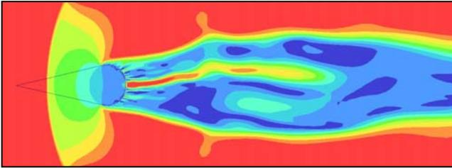
**Figure 18. Fluid Flow Through an Inflated Ribbon Parachute**
