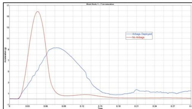
**Figure 8. Vehicle Vertical Acceleration of Similar Generic Spacecrafts with and without Airbag Attenuation**
