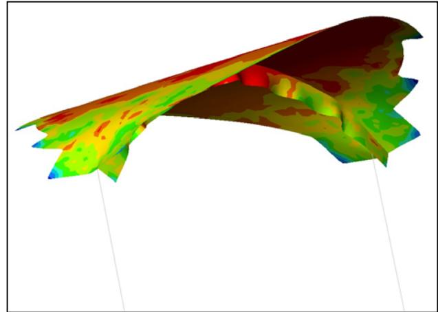
**Figure 1. Door Ejection Result – Deformed Shape Due to Thrusters**
