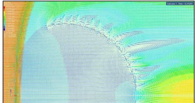
**Figure 16. 2D Flow Field through Rigid Representation of a Ribbon Parachute**
