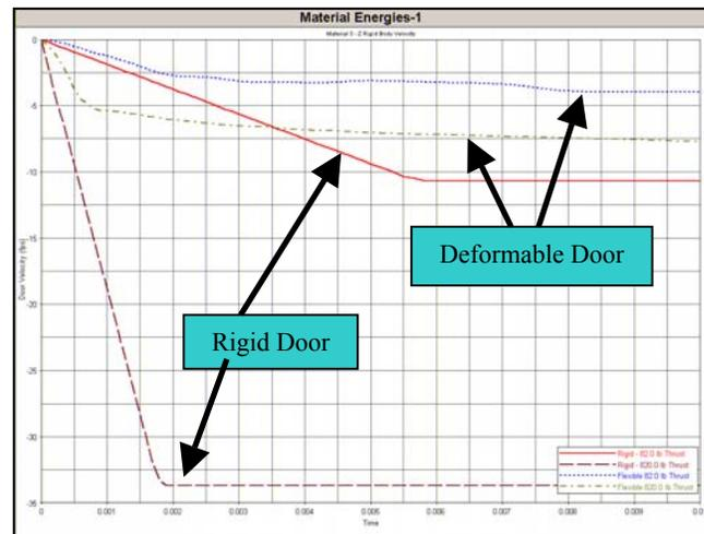
**Figure 2. Door Ejection Result – Door Velocity, Rigid Versus Deformable**
