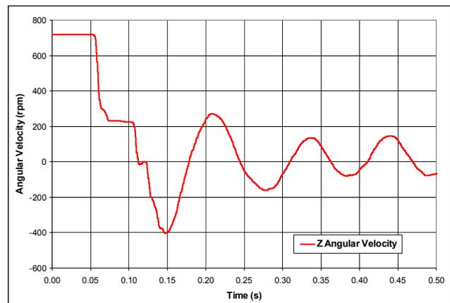
**Figure 10. Z Axis Rotational Velocity – Shows Arrest and Counter Rotation of the Fore Body**
