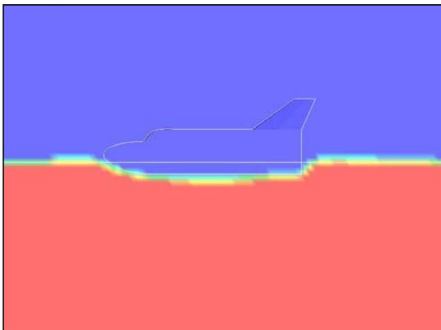
**Figure 6. Nominal Landing of a Generic Spacecraft into Water**
