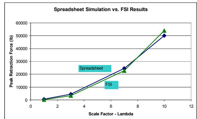
**Figure 15. Same Multi-body Simulation – Parachute Air Mass Adjusted to Match FSI Result – Same Volume Formula Used for all Scale Factors**
