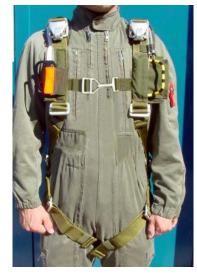
Operation is by static line or manual ripcord. The integrated SAVA device introduces a time delay between static line or ripcord operation to ensure that the parachutist is at a safe height and speed prior to canopy deployment. An emergency oxygen bottle is contained within the pack for high altitude escape. An override emergency ripcord will allow the parachutist to deploy the canopy independently of the SAVA mode of operation.
