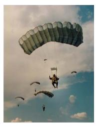
The MT-1 Series offers a full range of tactical parachutes for Special Operations, HALO, and HAHO missions. The parachutes were specifically designed and engineered for tactical military operations. The systems have been live tested at altitudes of up to 35,000 feet (10,668 meters) and use gliding parachutes in both the main and reserve compartments. There are a number of available main canopies and reserve canopies, as well as harness/containers to accommodate various combinations.
