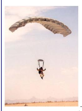
The MT-1Z main canopy is a ram-air pressurized gliding parachute designed specifically to improve the offset distance capabilities of tactical gliding parachute systems. It is an 11-cell canopy, which comes in two sizes: 308 ft<sup>2</sup> and 370 ft<sup>2</sup>.
