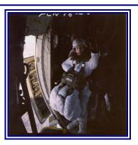
NATO STOCK NUMBER: 1670-00-262-2359 PART NUMBER: 11-1-900-2 **ASSEMBLY WEIGHT:** 13 KG (29 LB) **CANOPY MATERIAL:** MIL-C-44378/PIA-C-44378 T1, Low Porosity Nylon **ALL-UP SUSPENDED WEIGHT (AUW):** 160 KG (350 LB) RATE OF DESCENT AT 90 KG AUW: 4.7 M/S (15.5 F/S) MINIMUM DEPLOYMENT ALTITUDE: 150 M (500 FT) AGL **MAXIMUM DEPLOYMENT SPEED:** 278 KM/H (150 KTS) FORWARD SPEED: 4.5 M/S (15 F/S) TIME FOR 360° TURN: 9 SECONDS AGE LIFE: 16.5 years
