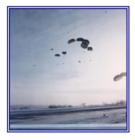
NATO STOCK NUMBER: PART NUMBER: ASSEMBLY WEIGHT: MINIMUM LOAD CARRYING CAPACITY: MAXIMUM LOAD CARRYING CAPACITY: (Cluster of 3 canopies) MINIMUM DEPLOYMENT ALTITUDE: 1670-00-999-2658 11-1-578 17 KG (37 LB) 45.5 KG (100 LB) 682 KG (1500 LB)
