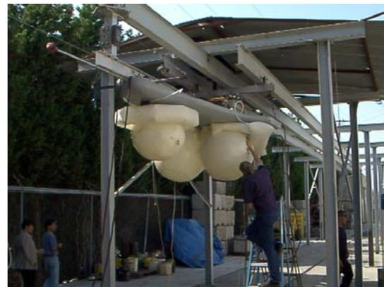
**Figure 11 – Airbag Drop Test Set Up**
