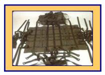
**THE A-22** assembly consists of a protective canvas cover, an adjustable nylon suspension sling complete with reinforced cotton duck scuff pad and a set of nylon suspension webs. A beveled plywood skid board is also available as an optional extra. Typical loads for the A-22 include rations, ammunition and liquid drums containing gasoline, oil and water.
