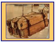
**THE A-7A** assembly consists of a set of 4 individual straps, each fitted with a permanently attached quick-fit fastener and a "floating" D-ring (removable). Each strap is manufactured from 1-3/4 in. (4.4 cm) nylon web, having a tensile strength of 6,500 lbs (2,955 Kg), and has a finished length of 188 in. (4.8 m). The A-7A may be assembled in various configurations of 2, 3, and 4 straps to rig such typical loads as jerry cans, fuel drums, ammunition, and other miscellaneous troop supplies.
