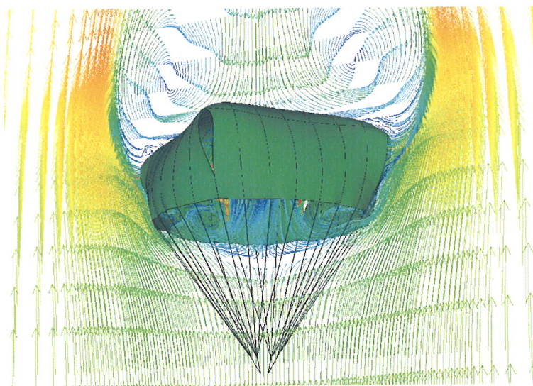
Figure 4. Velocity vectors on a section plane through the XT-11.
